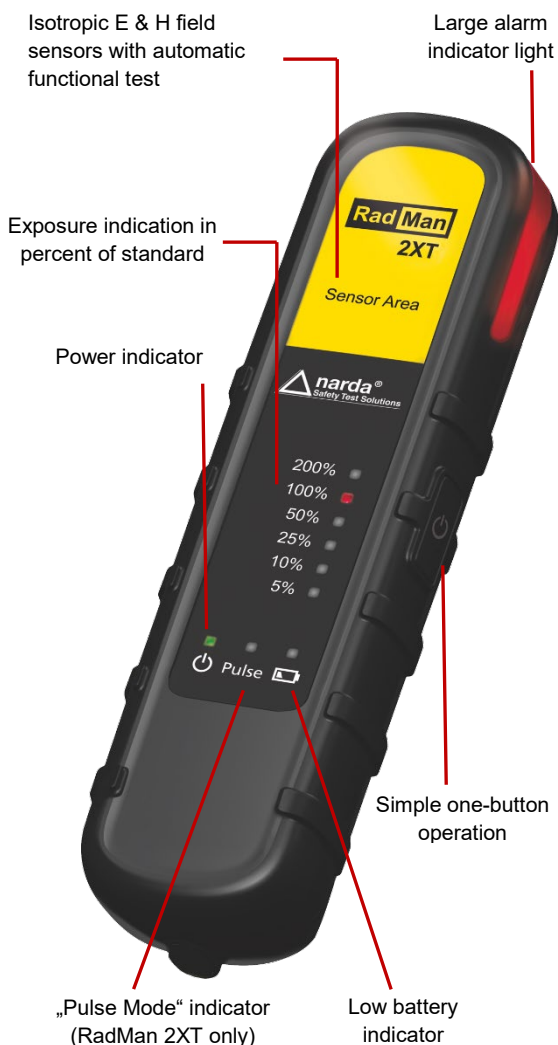
Fig. 1. Front view with controls and indicators
